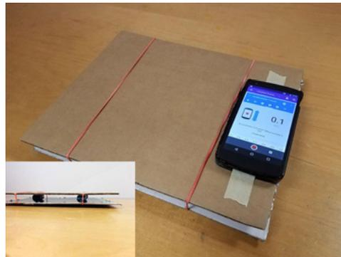
Make sure the Science Journal app is measuring acceleration in the appropriate direction and give it a test. You should be able to get at least 6 m/s<sup>2</sup> (meters per second squared) worth of vibration from your simulator.
